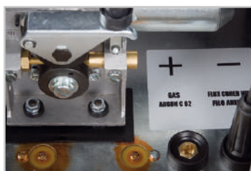
Polarity inversion for the use of flux core wires with the KOMBI 171 ED
