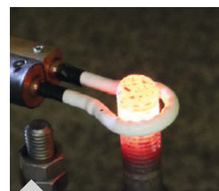
Heating a threaded bolt with the liquid-cooled coil
