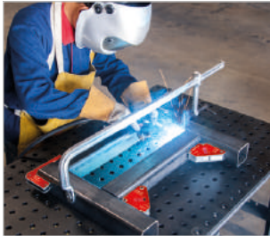
For holding metal workpieces at 45° or 90° angles
