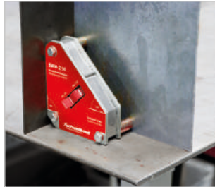
For holding metal workpieces at 45° or 90° angles
