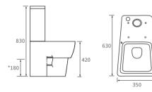
Coupling to soil stack: Horizontal or Vertical Distance from soil pipe spigot to wall: 225mm Cistern inlet position: Left
