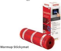
The Warmup StickyMat consists of a thin loose wire evenly spaced and taped to sturdy glassfibre mesh with pressure sensitive adhesive. It allows for the fastest and most secure installation of electric underfloor heating. Simply roll out a length, cut, flip and stick down the mesh until the floor area is covered. It is perfect for evenly heating large or regular-shaped rooms.
