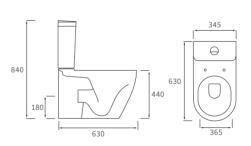
Coupling to soil stack: Horizontal and Vertical Distance from soil pipe spigot to wall: 210mm Cistern inlet position: Left and Right
