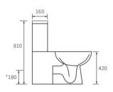
Coupling to soil stack: Horizontal or Vertical Distance from soil pipe spigot to wall: 220mm Cistern inlet position: Left
