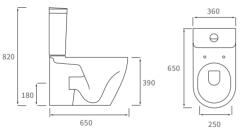
Coupling to soil stack: Distance from soil pipe spigot to wall: 225mm Cistern inlet position: Left
