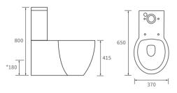
Coupling to soil stack: Horizontal Distance from soil pipe spigot to wall: 225mm Cistern inlet position: Left
