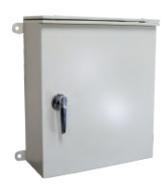
To improve the reliability of equipment operation, we provide an integrated intelligent solar monitoring box which consists of SPD (Surge Protection Device), No Fuse Breaker(NFB), AC switch, gateway, AC/DC converter and 110V/220V power outlet. The solar communication box is IP55 graded, waterproof, dust resistant and equipped with door lock that meets the specification requirement of all major solar power plants.
