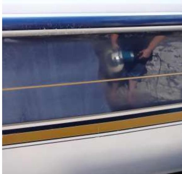
Only apply light pressure when compounding. Gelcoat will burn if your buffer speed is too high and/or if you apply too much pressure or product. Take your time and let the machine and product do the work. Use an air compressor to blow compound dust from the interior before proceeding. It gets easier after you have a few feet completed.
