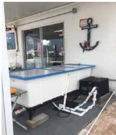
A new bait tank was installed at the Marina in June to improve the stability in the tank to keep more shrimp alive with the new water chiller.
