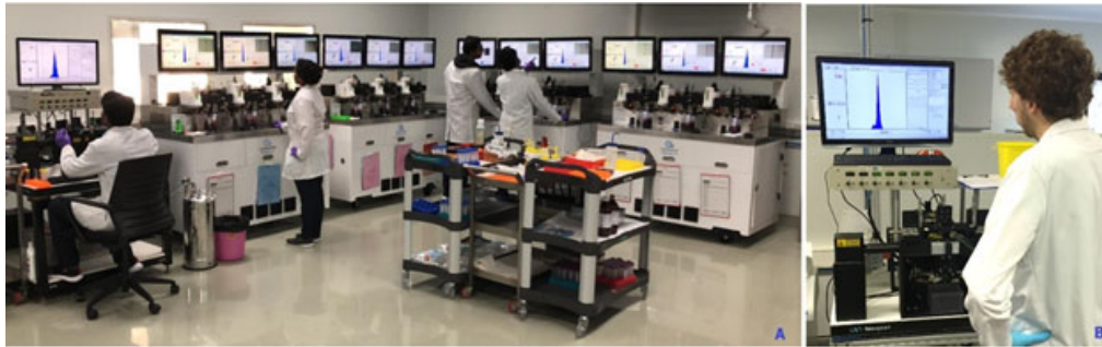
Figure 5. Use of Genesis™ high-resolution flow cytometry allows precise targeting of Sexed ULTRA™ gender purity. High-resolution flow cytometry is used throughout the production process to ensure sorting equipment are properly calibrated and setup (A: note Genesis 1 analyzer on the left being used in a production laboratory). High-resolution flow cytometry is also used as part of the quality control process to ensure minimum gender purity on all approved semen batches (B).
