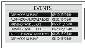
Use the press buttons and to scroll through the different screen and access the EVENT screen where 150 of the latest events can be found.
