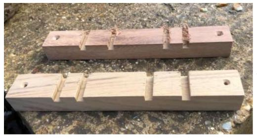
The sleepers come out with all slots milled in the correct positions. The photo shows how they come off the 'gang router' (rear sleeper) and final cleaned up and ready for use (front sleeper).
