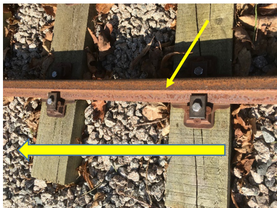
Figure 8: Witness mark on outside edge of left rail. Arrow shows direction of travel.
