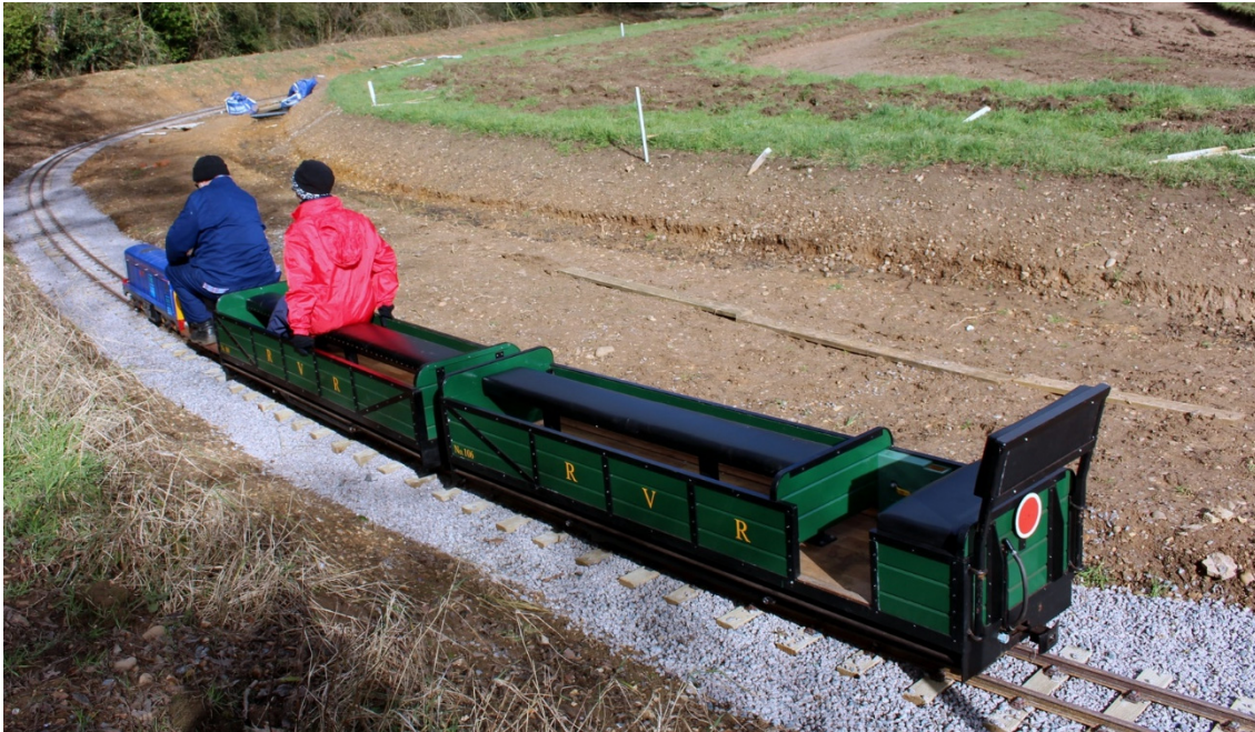
Figure 3: The train formation with "Class 20" battery electric loco, driving truck and standard Series 100 coach pair.
