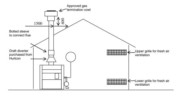
A Hurlcon indoor draught diverter must be fitted to unit in accordance with Hurlcon's Instructions and Installation Codes before the boiler can be enclosed.
