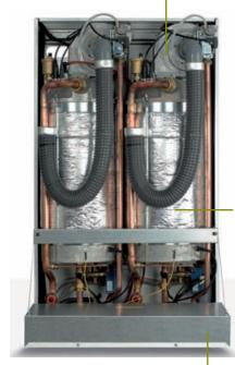
High efficiency 50 kW heat exchanger consisting of a continuous bimetal corrugated helical tube (copper on the water side and AISI 316 stainless steel on the flue side). The micro flame steel burner is located in the upper part of the heat exchanger with single spark ignition.
