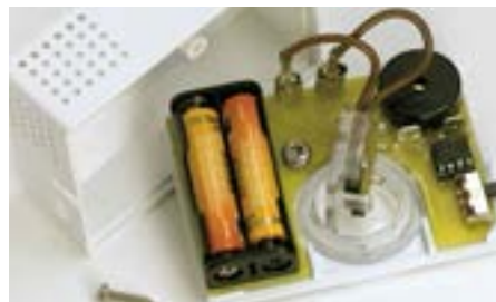
Insert the batteries (not supplied) into the case
