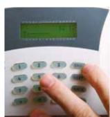
SECURITY SYSTEM COMPATIBLE B&D Openers are able to be wired to alarm systems. This allows your handheld opener transmitter to arm and disarm the alarm.
