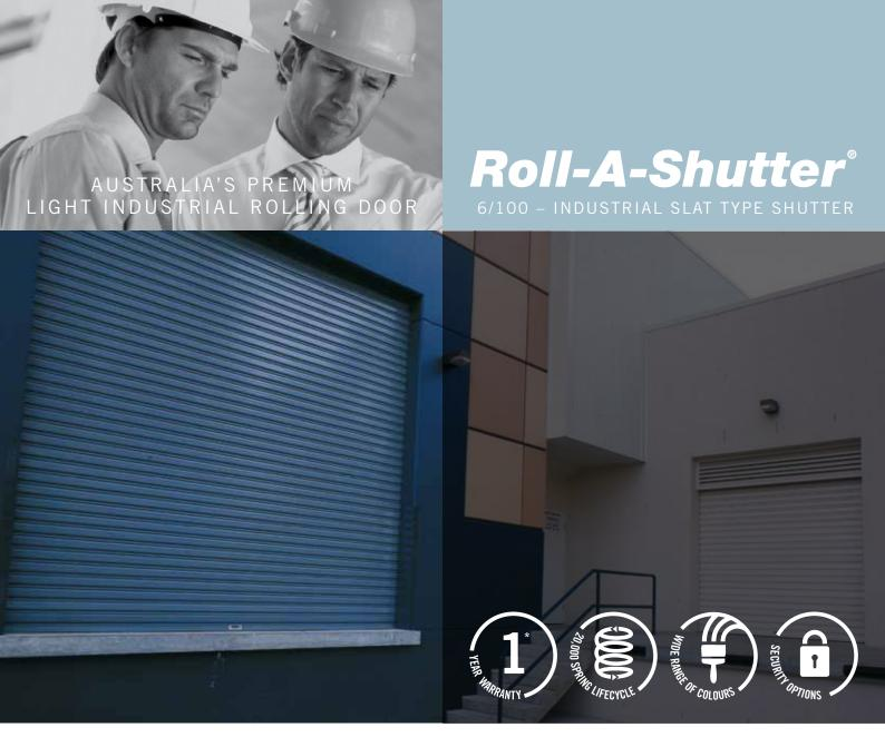
The 6/100 Roll-A-Shutter curtain is made from 0.6mm thickness continuous roll formed interlocking type coated galvanised steel slats, having a nominal effective pitch of 100mm and a zinc coating of not less than 250g/m².
