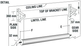
"E" = measurement from end of drum (not the gear wheel) to the fixing bolt centre line. Gear side.
