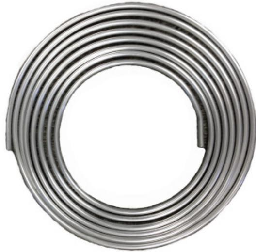
Cost effective seamless aluminum tubing can be used to form O.E. type fuel, water, oil supply lines. Use with AN818 tube nuts and 819 flair tube sleeves or compression hard tube adaptors.
