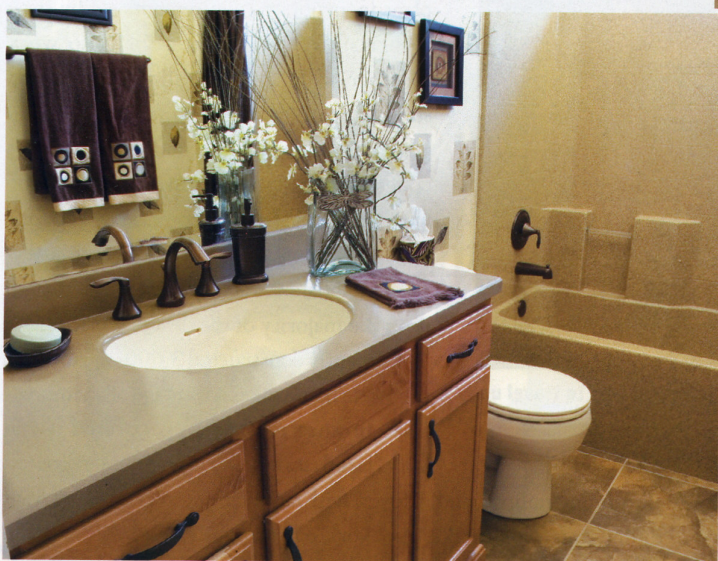
Below: One would think that this tub and shower was made of Corian or granite. However, it is actually a fiberglass insert with a special glazed finish. The countertop sitting on the maple cabinet is actually Corian.
