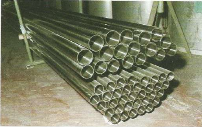
Tubi Ø 34 e 70 mm lucidati interno ed esterno Tubes Ø 34 and 70 mm. Processing: Internal and external lustre polishing
