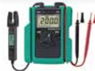
Multi Tester Digital - TAS00021 DC Volt : 340 Mv / 3.4/34/340/600 V AC Volt : 3.4/34/340/600 V Resistensi : 340Ω/3.4K/340K/3.4M/34M Ω Konduksi : Buzzer sounds when 30 ± 10 Ω or less Frekuensi : (Current) 3.4 k / 10 kHz (voltage) 3.4 k / 34 k / 300 kHz Batteries : AAA batteries R 03 (1.5 V) x 2 - W 87 x D 21 x H 128 mm - about 210 g
