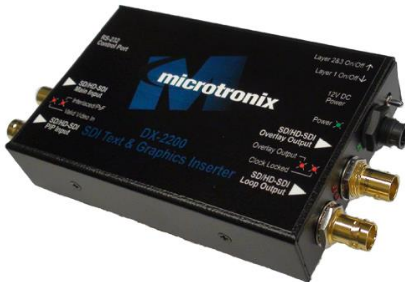
Figure 2: DX-2200-TI-24 – SD/HD-SDI Text & Graphics Inserter with PIP and SDI Loop Output
