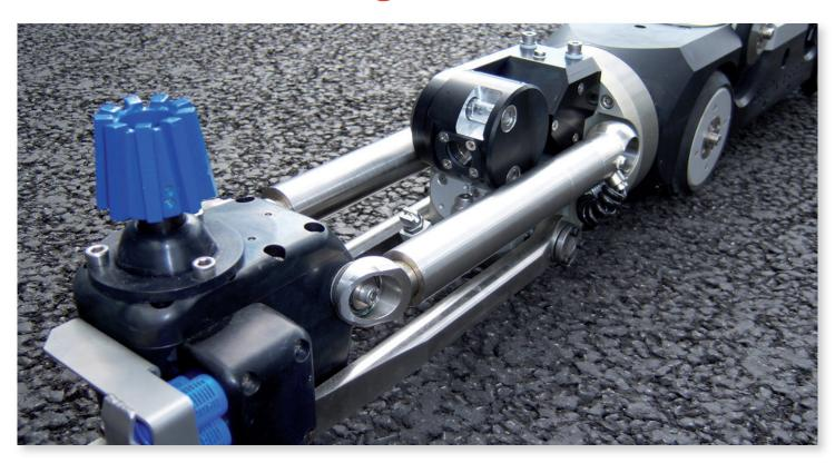
Lateral preparation and re-opening cutting is a critical part of any sewer rehabilitation project as the relining itself. Therefore all of it must be fit for purpose.
