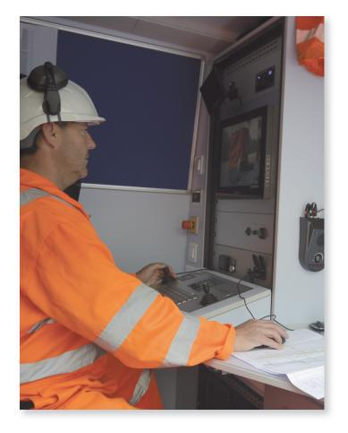
With on-site vehicle broadband connections, immediate survey reports in a PDF format can be sent to your desk for instant decision making. Using Wincan mobile software on site, allows for first hand accuracy in formulating surveys in Wincan code. Doing so, eliminates the risk of office based errors.
