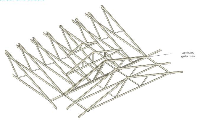
The girder and saddle truss eliminates the need for a load-bearing wall at the intersection of two gables in the roof structure.
