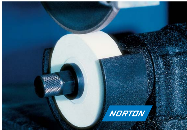
AFTER DRESSING THE WHEEL FACE IS OPEN WITH THE GRITS EXPOSED, READY FOR EFFICIENT GRINDING ACTION
