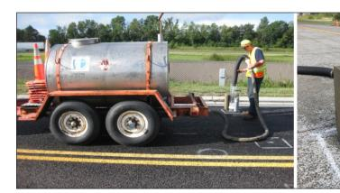
Permeability tests in which water is flushed through the pavement structure were central to the investigation of porous asphalt pavements. The tests confirmed that porous asphalt drains and filters water effectively through the pavement structure.
