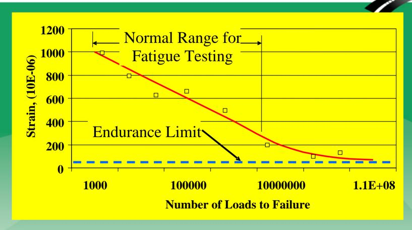
Normal Fatigue Testing Results Versus Endurance Limit Testing
