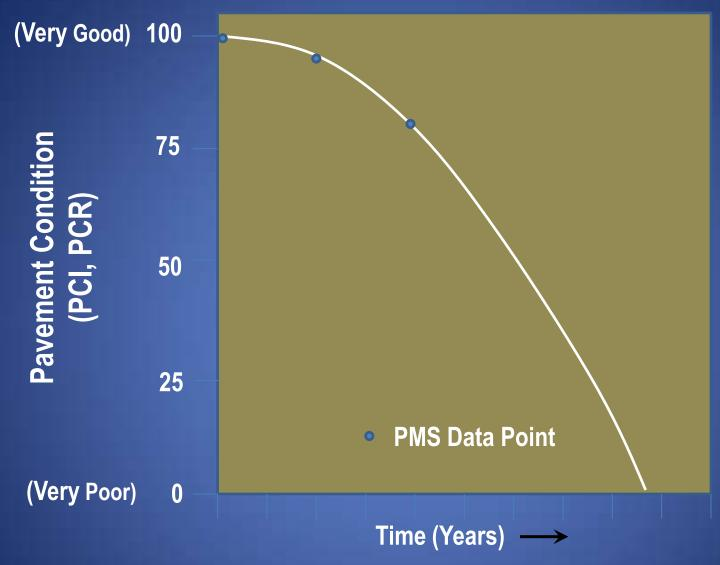
Pavement Condition Index (PCI) and Pavement Condition Rating (PCR) are widely accepted pavement rating systems.
