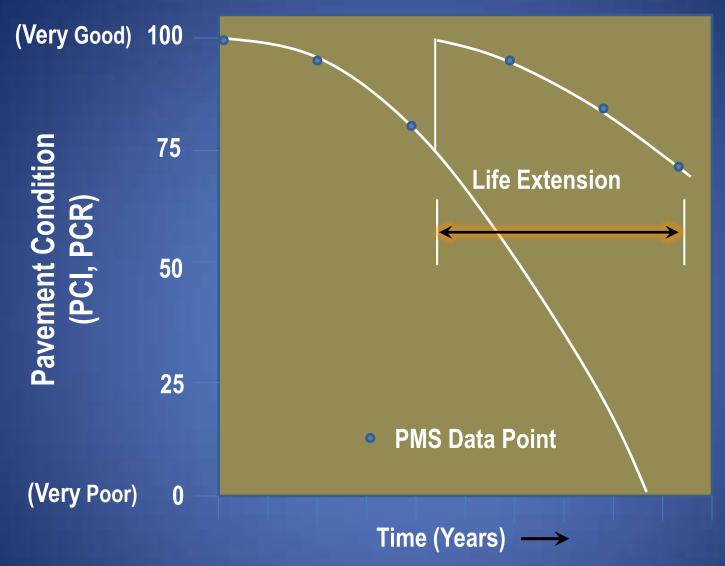
Life Extension depends on (1) structural soundness of the pavement upon which the preventive maintenance treatment is to be applied, and (2) robustness of the treatment.
