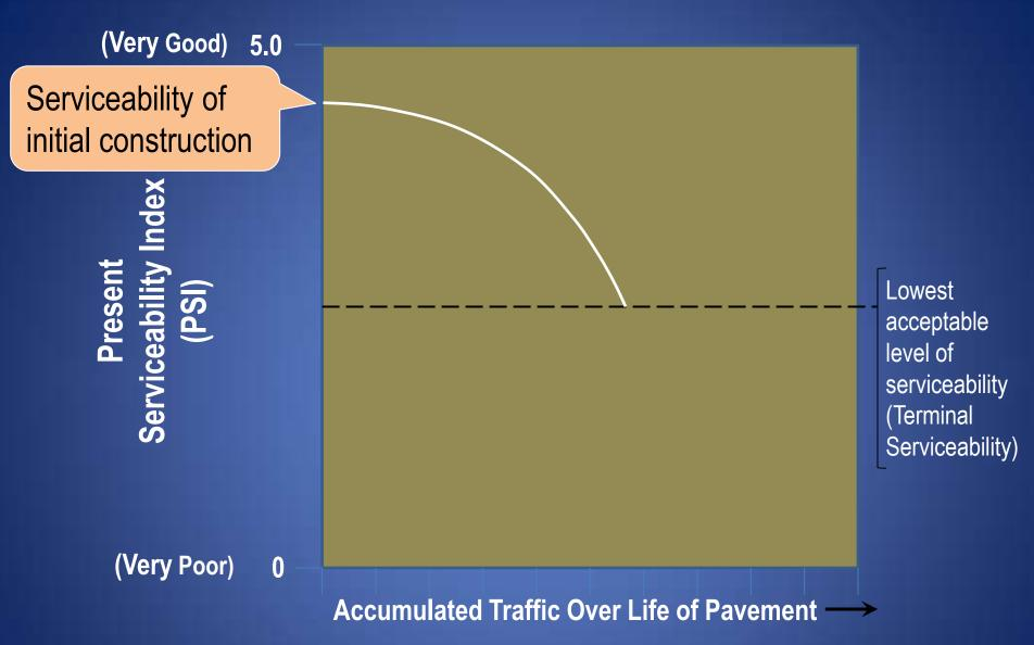
Serviceability declines as a pavement deteriorates under the punishment of traffic. The lowest tolerable level of serviceability is called the "Terminal Serviceability".
