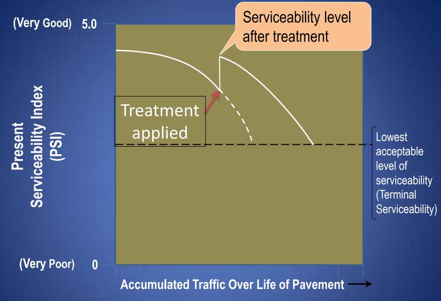
Preventive maintenance treatments arrest the deterioration in service caused by traffic. Serviceability is restored to a level commensurate with the treatment type.
