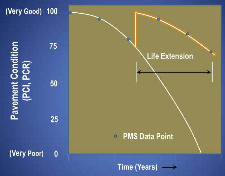
With the application of a preventive maintenance treatment pavement distresses are corrected and condition is improved. Pavement life is extended.
