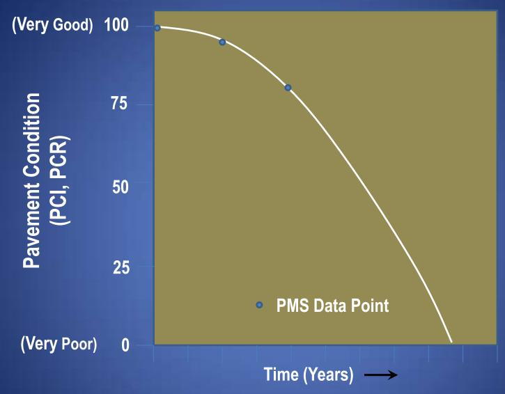
Pavement condition is assessed on a scale of 0 to 100, where a rating of 100 indicates no distress exits or, in the case of a pavement rehabilitation, all distresses have been corrected.
