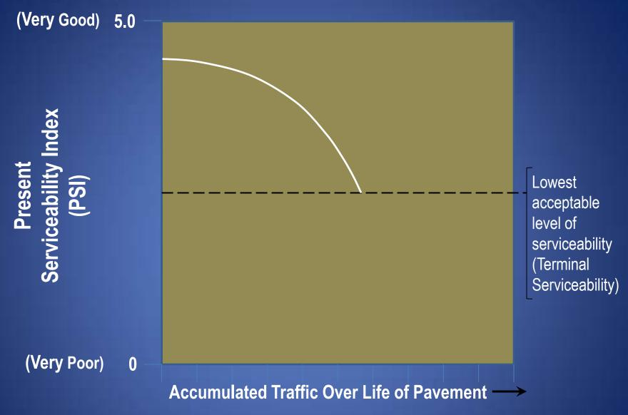
Present Serviceability Index uses a rating scale of 0 to 5, with 5 indicating the highest level of acceptability to the user.
