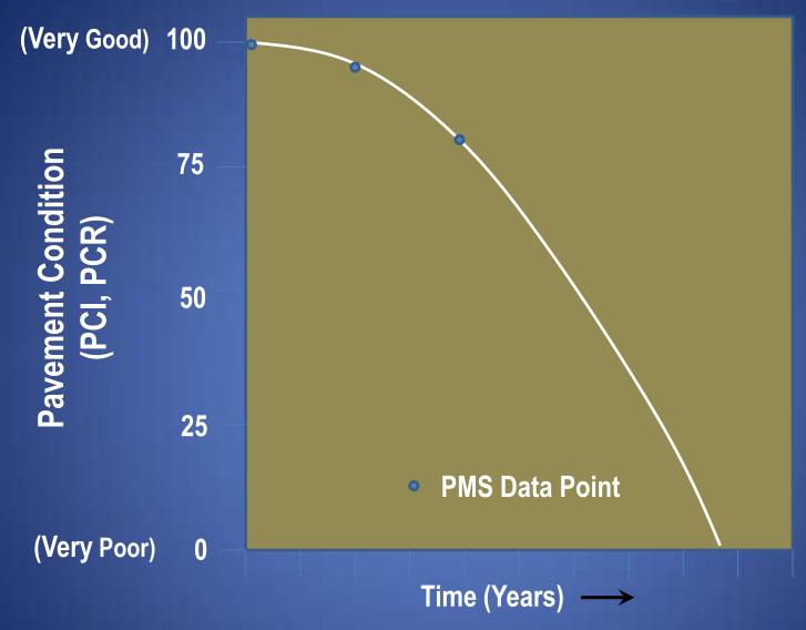
The plot of pavement management system (PMS) data indicates the rate of deterioration in pavement condition as determined by measuring severity and extent of pavement distresses.
