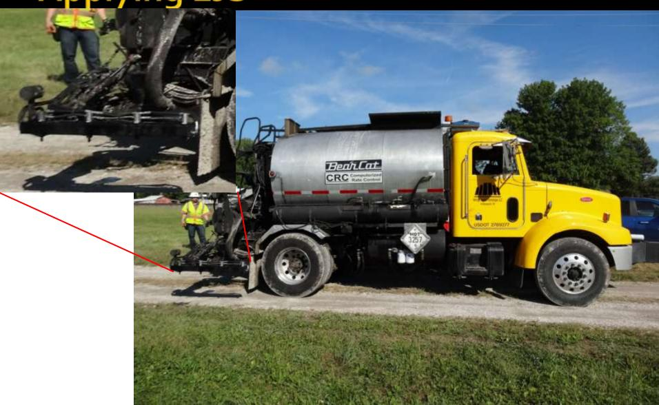
Heavy Duty Pressure Distributor for Applying LJS
