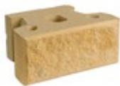
Standard Unit Size: 455 L x 315 W x 200 H mm Weight (each): 41 kg Face area: 11 units per m 2
