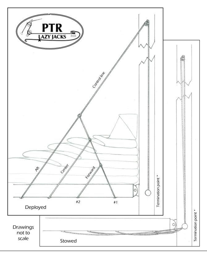
Lazy jacks are designed to contain the mainsail when reefing or dousing. PTR Jacks are easy to deploy and stow with no parts or lines that are subject to or cause chafe. We offer standard and off-shore options dependent on your sailing goals. Our system has Amsteel catch lines and double braid control lines. The kit includes blocks and fasteners. No modification of your sail cover is required.
