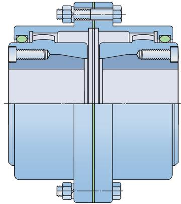
Gear coupling mounting
