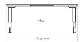
Table Top Depth Minimum: Rated Input: 207-253V/50-60Hz 750mm Feet Depth: Rated Output 230V/50Hz 750mm 0.3W Maximum Speed: 36mm/sec Power Consumption (Standby) Frame Load Maximum: 120kg Equally Divided Power Comsumption (In Use) 216W
