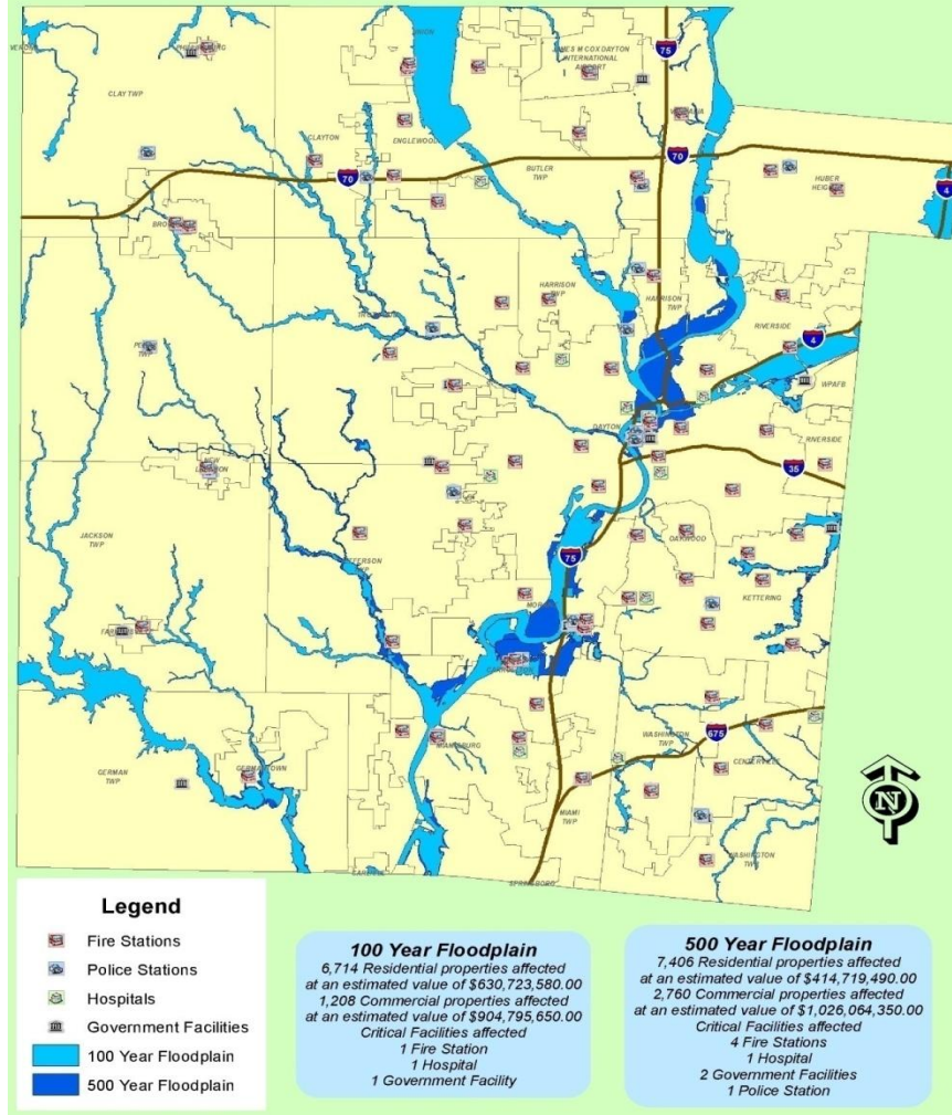
• Figure 4-5: Structures in the Special Flood Hazard Area
